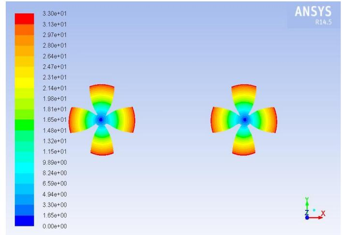
Figure 4. Velocity contours of the propellers
