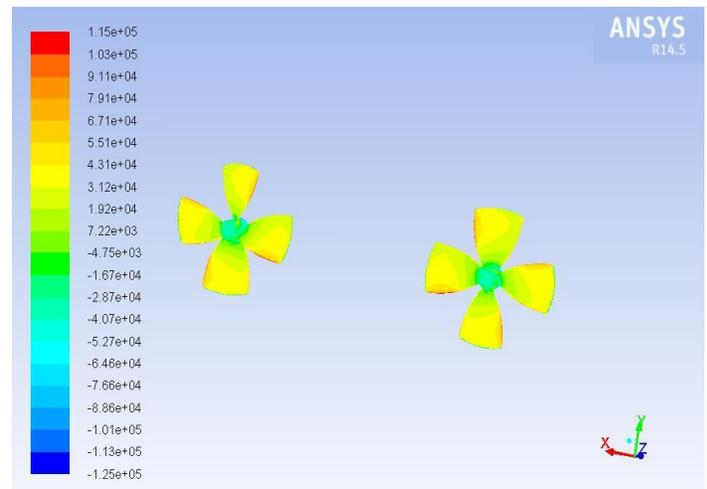
Figure 5. Pressure contour of the suction side
